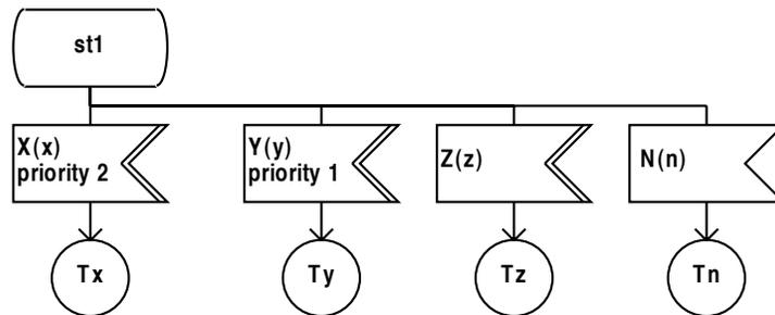
Fig. 6. Multiple levels of input priority
