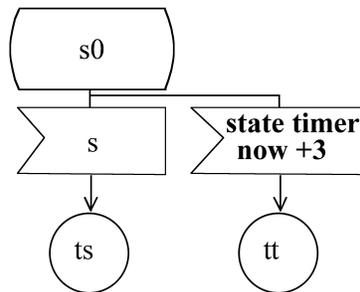
Fig. 7. Timer supervised state with an implicit timer
